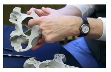
A model of an elephant's skull made with a 3-D printer by students in Professor Lorna Gibson's *3.054 Cellular Solids: Structure, Properties and Applications.*
