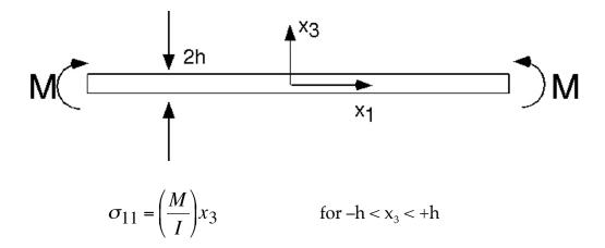
M is the bending moment (which is constant in  $x_1$ ), and I is the second moment of area of the cross-section of the beam (which is also constant). If  $\sigma_{12} = \sigma_{32} = \sigma_{22} = \sigma_{33} = 0$  what can you say about the variation of the shear stress  $\sigma_{13}$  with  $x_1$ ,  $x_2$  and  $x_3$ ?
