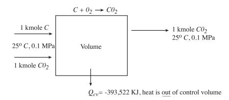
Figure C-1: Constant pressure combustion
