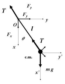
There are two forces acting on the suspended mass: the string tension and the weight. By our earlier argument, the tension, T, is parallel to the position vector r and therefore its moment about O is zero. On the other hand, the weight creates a moment about O which is  $M_O = -lmg \sin \theta k$ . The angular momentum is given by
