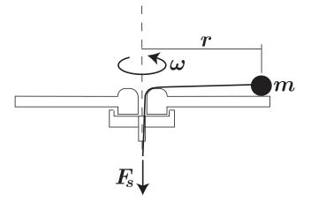
The component of the moment of the forces acting on the particle is zero along the spinning axis. Therefore, the vertical component of the angular momentum will be constant. For i), we have
