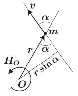
It is clear from its definition that the angular momentum is a vector which is perpendicular to the plane defined by r and v. Thus, on some occasions it may be more convenient to determine the direction of  $H_O$  from the right hand rule, and its modulus directly from the definition of the vector product,
