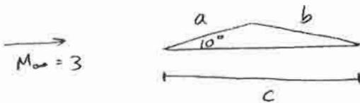
a) Approach: since pressure on lower surface is  $p_{\infty}$  according to shock-expansion theory, just need  $p_a, p_b$ .
