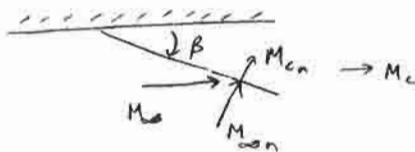
We know  $M_\infty$ , the normal Mach no. before the shock. Using normal shock relations, we can find  $M_{\infty n}$ , and then use trigonometry to get  $M_c$ .
