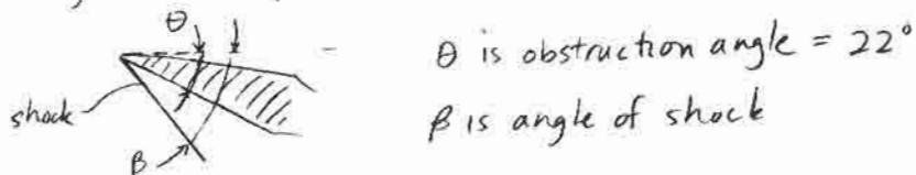
To get  $P_c$ , need the normal Mach number, since it controls the "jump" in flow properties. "Normal" means perpendicular to the shock (use  $\beta$ , not  $\theta$ ).
