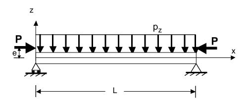
(a) Determine the individual contributions to the primary bending moment of the transverse load  $p_z$  and the off-axis application of the end load.
