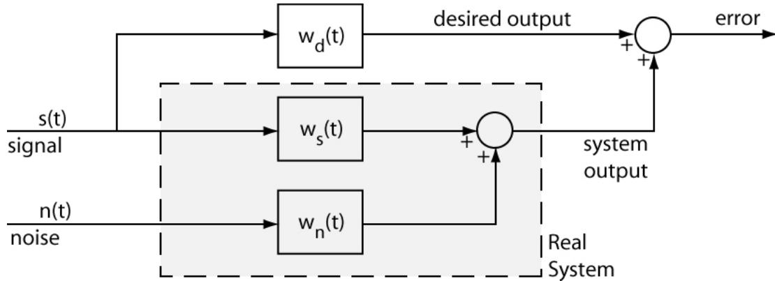
System parameters are contained in  $w_s(t)$  and  $w_n(t)$ .
