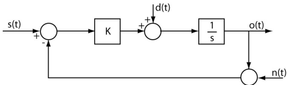
Signal  $s(t)$  is a member of a stationary ensemble:  $S_{ss}(\omega) = \frac{A}{\omega^2 + a^2}$
