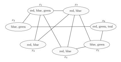
Draw the search tree of the backtracking algorithm and number the nodes according to their order of expansion until the algorithm finds a feasible assignment that solves the constraint satisfaction problem. The algorithm picks the colors according to the following order: blue, green, red, teal. Assume that the algorithm traces the variables according to the following order:  $x_1, x_2, x_3, x_4, x_5, x_6, x_7$ .
