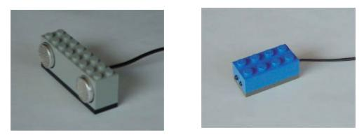
Figure 2 – Ultrasonic range sensor (left) and infrared proximity sensor (right)
