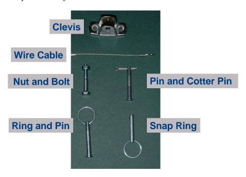
Figure 1 – Mechanical Assembly for Sailboat Rigging
