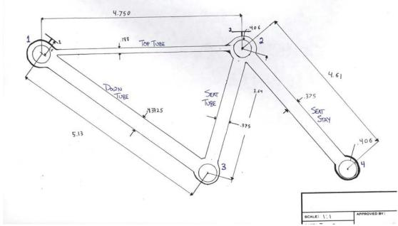
Beam 1 (top tube) is designed much narrower than Beam 2 (down tube) since it principally supports only the horizontal load at axis 1, which is smaller than the vertical loads at axes 1 and 2; Beam 2, oriented roughly at a 45-degree angle must support both the horizontal and vertical loads at axis 1.
