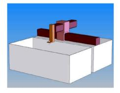
Floor-mounted cantilever system with separate cutting table
