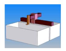
Adv: Less floor space is required for a given table size because the external support frame is eliminated
