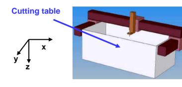
Floor-mounted gantry with separate cutting table
