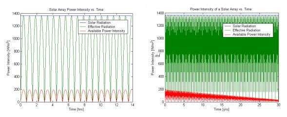
Figure 4. Solar array power intensity for a simulated low Earth orbit without an eclipse.
