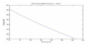
The function RTGPower.m exhibits exponentially decaying power, as expected of a radioisotope thermoelectric generator.
