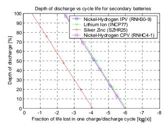
Figure 3. Relationship between depth of discharge and reduction in lifetime for chemical batteries.
