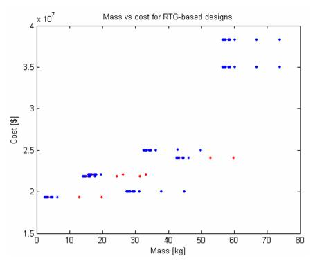
Figure 9. Mass and Costs for Design vector according to the input Power profile for an RTG source system
