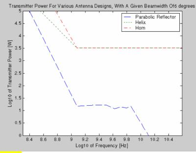
**Figure ?.** Relation Between Transmitter Power And Frequency (For A Given Beamwidth)
