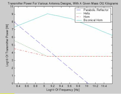
**Figure ?.** Relation Between Transmitter Power And Frequency (For A Given Mass)
