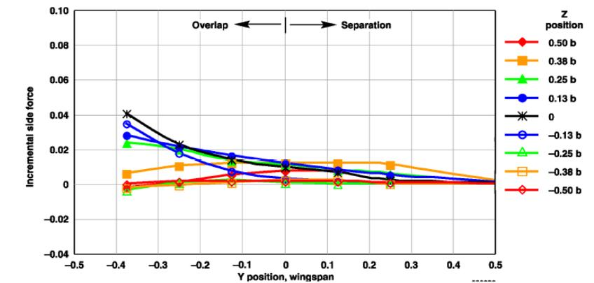
Vortex effects are weaker at transonic than at subsonic conditions
