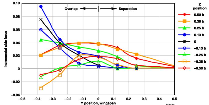
Peak vortex effects are coincident with the position for maximum drag reduction! 😊
