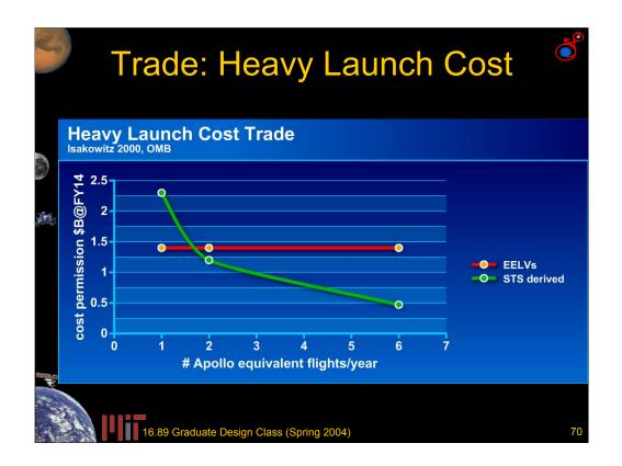
This graph shows the cost per flight of a whole Apollo class mission (short stay) to the moon. It compares two approaches one using many heavy EELVs (Delta-IV Heavy) to launch the mission in chunks, the other sending the astronauts in a separate EELV and the cargo on a Heavy STS derived.
