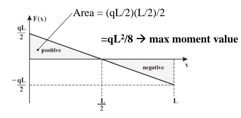
Shear diagram equals the slope of moment diagram
