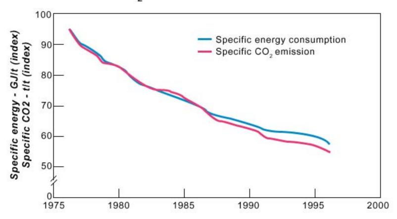
EU steel industry consumption per tonne of hot-rolled steel EU Steel Industry CO<sub>2</sub> emission per tonne of hot-rolled steel (3 year moving averages)
