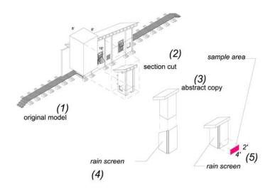
Figure 1. Process of reduction from starting building shape to CNC sample area
