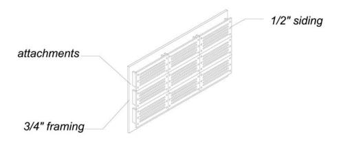
Figure 3 3D assembly of siding with backer board.
