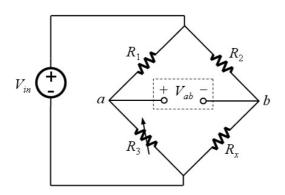
Figure 1: A Wheatstone bridge circuit.
