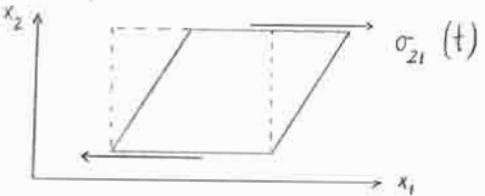
$$\begin{aligned}\sigma_{21}(t) &= 2 \int_{-\infty}^t G(t-\tau) \frac{d\varepsilon_{21}(\tau)}{d\tau} d\tau \\ &= 2 \int_{t_0-\xi}^{t_0} G(t-\tau) \frac{\varepsilon_0}{\xi} d\tau \quad \text{for } t \gg t_0 \\ &= 2 G(t - (t_0 + \xi)) \frac{\varepsilon_0}{\xi} \quad 0 \leq \xi \leq 1\end{aligned}$$
