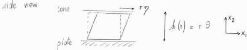
impose oscillatory shear  $\varepsilon_{21} = \frac{1}{2} \frac{\partial u_r}{\partial x_2} = \frac{1}{2} \cdot \frac{\pi \gamma}{\pi \theta} = \frac{\gamma}{2\theta}$  independent of radius
