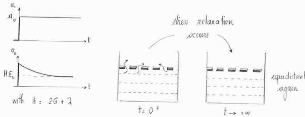
Impose step displacement  $u_0$  at  $t=0^-$ , and find  $u_i(x_i, t)$
