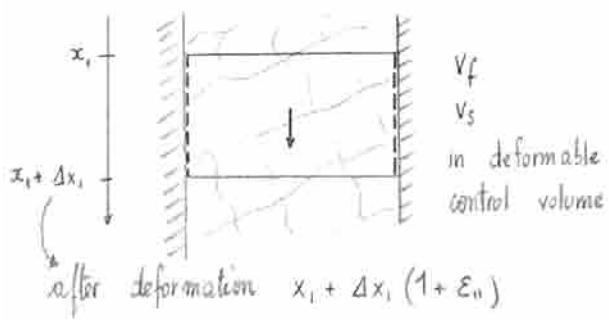
$$\text{net flux} = A_f (v_f - v_s)_{|x_i} - A_f (v_f - v_s)_{|x_i + \Delta x_i}$$
