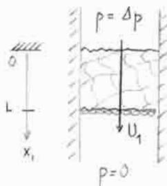
apply  $\Delta p$ , measure  $U_1 = \frac{\text{flow rate}}{\text{total area}}$
