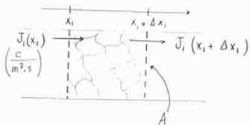
flux of charge into the element in  $\Delta t =$
