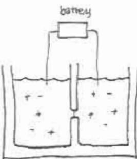
2 salt water chambers, hole ( $\sim \frac{1}{2}$  mm in diameter)
