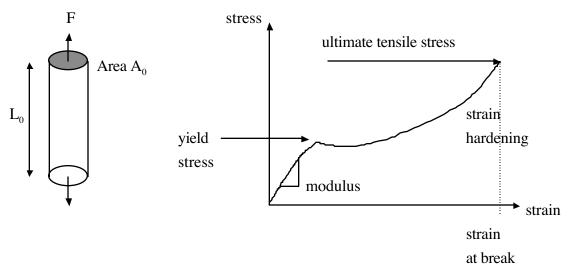
Figure: Schematic illustrating the tensile test and features on a stress-strain plot.
