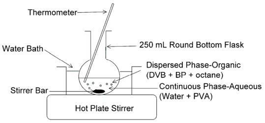
Figure: Experimental setup for Part B
