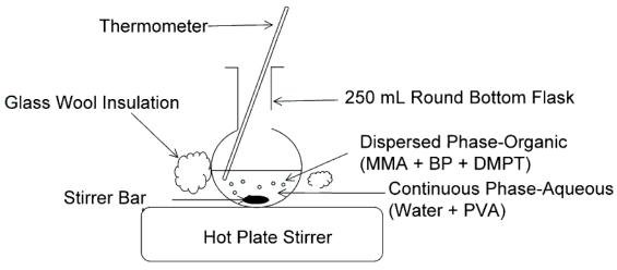
Figure: Experimental set up for part A
