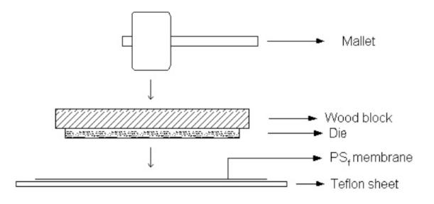
Figure 7: Using the die to cut the membrane
