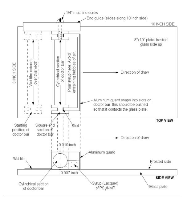
Figure 5: Membrane casting apparatus
