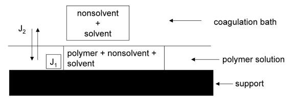
Figure 2. Schematic representation of processes after immersion in a nonsolvent bath;  $J_1$ : nonsolvent flux,  $J_2$  solvent flux
