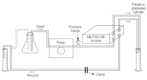
Figure 9: Final set up for permeability studies
