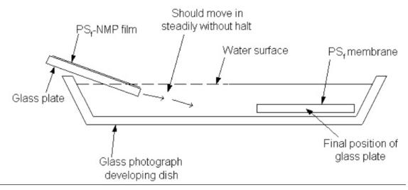
Figure 6: Immersion of the glass plate into the water bath
