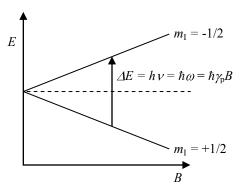
The NMR spectrum is an RF absorption spectrum. The magnetic field magnitude *B* is held fixed, but instead of scanning the RF frequency and recording how much RF power at each frequency gets through the sample, like in UV-VIS spectroscopy, the spin response is measured in the time domain. A short RF pulse is incident on the sample, inducing coherent oscillations of the spin magnetic moment which
