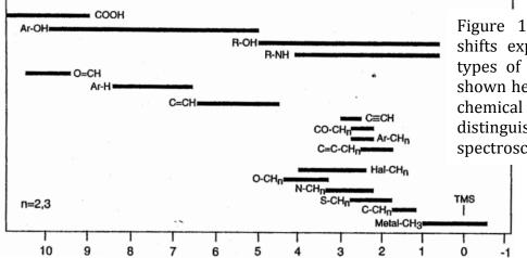
Figure 13. The chemical shifts expected for various types of <sup>1</sup>H resonances. As shown here, a wide range of chemical groups may be distinguished through NMR spectroscopy.
