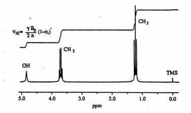
12. Figure The proton NMR spectrum of ethanol. TMS (the most widely used reference signal) stands for tetramethylsilane  $(Si(CH_3)_4)$ . The upper step-like curve is the integrated signal, proportional to the number of spins contributing to each set of peaks. From J.T. Arnold et al, Journal of *Chemical Physics* **19**, p. 507 (1951).
