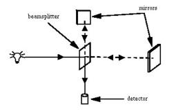
Figure 9: Interferometer (image from NIST, National Institute of Standards and Technology). For another example of an Interferometer, please see http://www.physics.mq.edu.au/ ~qoldys/optmicroweb/ftir
