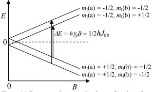
So, the effect of one nearby proton is to split the NMR absorption line into two closely spaced lines of equal intensity. If we extend this treatment to include another proton c that is indistinguishable from b (e.g. on an ethylene group) and that therefore interacts in the same way as b with
