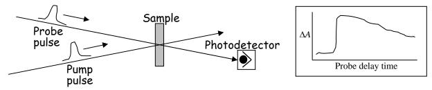
This can be done on femtosecond, picosecond, nanosecond,..., many-second time scales. The probe pulse absorption is changed by the pump pulse because the excited states and ground states absorb differently.
