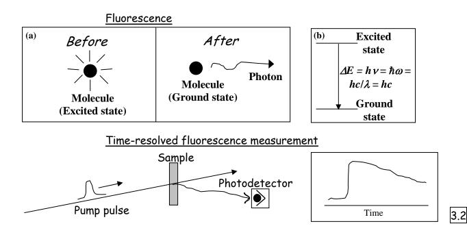
Fluorescence emerges in all directions. Some reaches the photodetector, producing a signal whose time-dependence is measured. As the excited molecules return to the ground state, the amount of fluorescence decreases.
