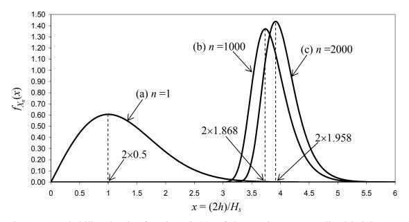
Figure 1: Probability density function,  $f_{X_n}(x)$ , of the maximum normalized height,  $X_n = (2H_n)/H_s$ , of *n* waves.
