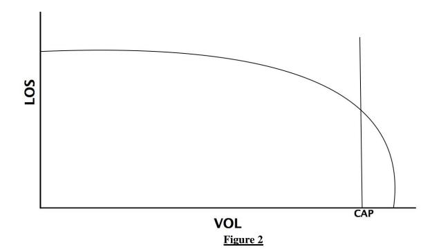
This is the characteristic hockey stick shape well known to transportation specialists. As VOL approaches the capacity (CAP), LOS deteriorates sharply. Going from a VOL of 80% of CAP to 90% of CAP can have a large detrimental effect on LOS.
