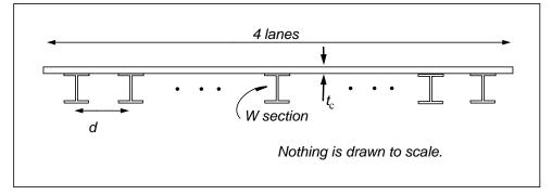
You are to first take the concrete and steel as acting independently. In fact, in this part you are to take the contribution of the concrete to bending strength and stiffness of the steel beams as nil.
