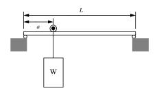
A simply supported beam (indicated by the rollers at the ends) carries a trolley used to lift and transport heavy weights around within the shop. The trolley is motor powered and can move between the ends of the beam. For some arbitrary location of the trolley along the beam, a,
