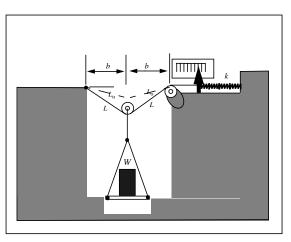
From equilibrium, letting *T* be the tension in the cable (not shown) we have  $T = \frac{W}{2\sin\theta}$ Compatibility yields  $\frac{\Delta}{L_o} = 2 \cdot \left(\frac{1}{\cos\theta} - 1\right)$ . where  $\Delta$  is the deflection of the spring, positive to the left in the figure<sup>1</sup>.
