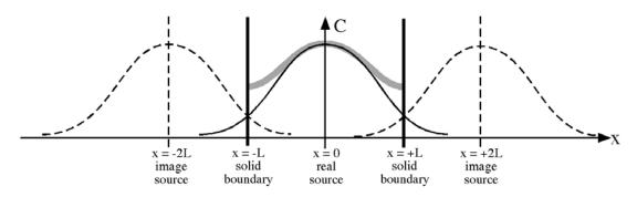
**Figure 3.** To satisfy the no-flux condition at both boundaries, two image sources (dashed) are added to the real source (black). For short time, the sum of these three sources (gray) is sufficient to satisfy  $\partial C/\partial x = 0$  at  $x = \pm L$ . However, at later time each image source will begin to lose mass across its opposite boundary, and the no-flux condition will no longer be satisfied. Ultimately, images will be needed at  $x = \pm 2nL$ , for all integer n.
