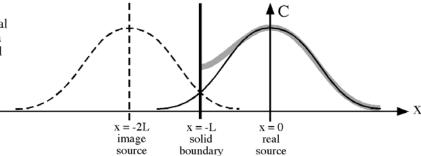
The superposition (sum) of the original and image sources is shown within the flow domain (x > -L) as a thick, gray line. Note, specifically that this curve satisfies the condition  $\partial C/\partial x = 0$  at x = 0, as stated in (6). The solution is thus the sum of (7) and (8),
