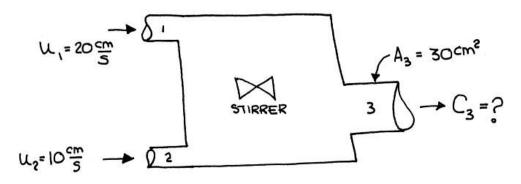
Two pipes, each of  $10 \ cm^2$  cross-section, carry water into a mixing chamber. The upper pipe carries water saturated in oxygen ( $C_1 = 9 \ mg/l$ ), and the lower pipe carries deoxygenated water ( $C_2 = 0 \ mg/l$ ). A stirrer within the chamber rapidly mixes the two streams, such that the concentration in the tank is spatially uniform. Assuming the system is at steady state, what is  $C_3$ ?
