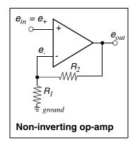
As an example of a single input application, consider the "noninverting amplifier" shown at the left. First some rules of behavior of our black box. Quoting The Art of Electronics:
