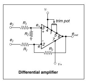
$e_{-} - e_{out} = \frac{R_2}{(R_1 + R_2)} \cdot (e_1 - e_{out})$  and since  $e_+ = e_-$ , we obtain, after some manipulation left
