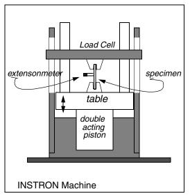
The output of the extensionmeter and the load cell will be automatically recorded on a pc. You are to make note of the load and displacement factors so that you can convert the voltage readings so recorded to force (then stress) and displacement (then strain). The original length between the points of attachment of the extensionmeter should also be noted.
