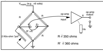
If available, use two voltmeters to measure both the input voltage to the op-amp  $e_1 - e_2$ , and the output voltage of the op-amp, pin 6 to ground. First, short out the input, connecting  $e_1$  and  $e_2$  using a short jumper wire. Then, adjust the 10 Kohm trim pot until the output of the op-amp is zero, i.e., within a few millivolts of zero. (Zero does not exist in the material world).
