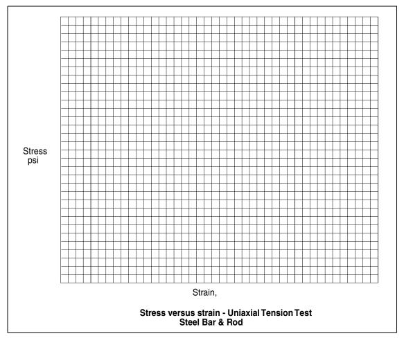
The slope of the stress/strain curve in the linear elastic range gives a value for the elastic modulus
