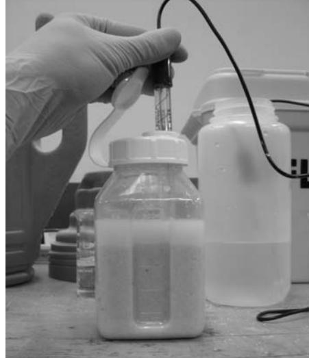
4. Begin Experiment: Have pH sensor ready. Add the acidic water until an excess of 1/2 inch of water exists above the material, as shown above left. Immediately begin measuring the pH in the layer of excess water above the grains. Insert the probe through the opening in the cap of the container, as shown above right. Remember, the sensor has a very thin glass membrane, so be careful to just insert it into the water and not the granular material.
