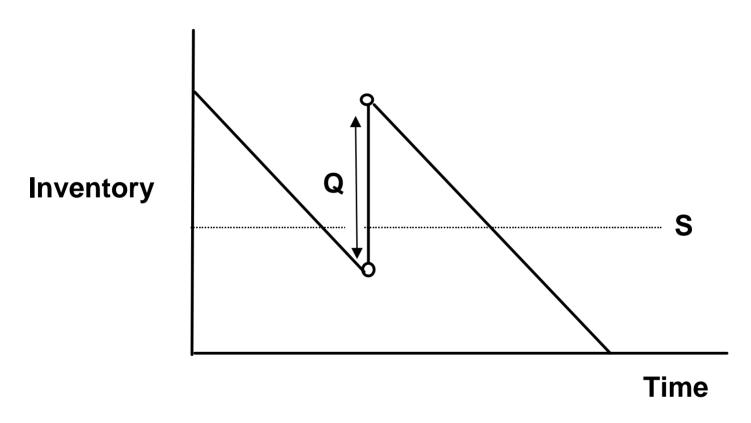
The operating rule is: When the inventory reaches 'S', reorder 'Q' items, where 'Q' is the reorder quantity.
