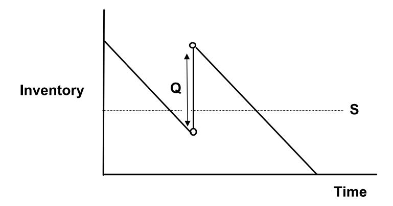
The operating rule is: When the inventory reaches 'S', reorder 'Q' items, where 'Q' is the reorder quantity.
