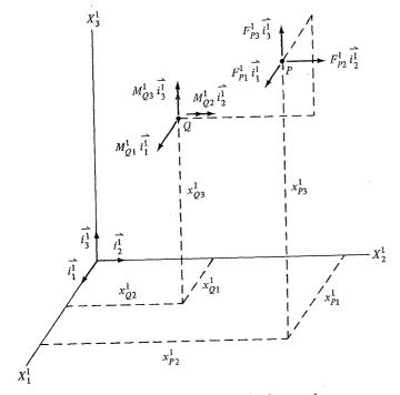
Fig. 5-3. Notation for orthogonal reference frame
