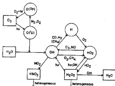
Fig. 1. Major chemical reactions affecting odd hydrogen (OH, H, HO<sub>2</sub>, H<sub>2</sub>O<sub>2</sub>) in the troposphere.
