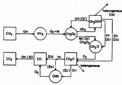
Fig. 2. The atmospheric oxidation of methane.
