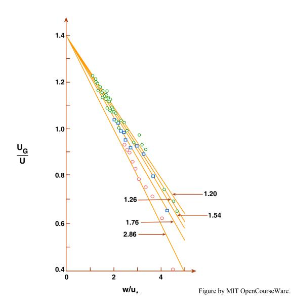
Figure 10-7. Plot of dimensionless particle speed  $U_G/U$  vs. the ratio of particle settling velocity to shear velocity,  $w/u_*$ . Different symbols and lines refer to experimental particles of different specific gravities. (From Abbott and Francis, 1977.)
