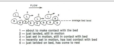
Figure 10-1. The flow, the bed, and the load.
