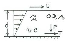
Figure 10-9. Variables governing dispersive stresses in a sheared sediment–fluid mixture, in the absence of gravity.
