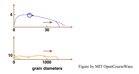
Figure 10-5. Sketches of typical particle trajectories observed by Francis (1973). Above: saltation trajectory. Below: suspension trajectory (wavy line, with saltation trajectory shown to same scale for comparison. (From Francis, 1973.)
