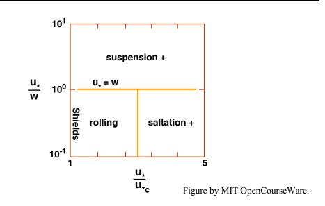
Figure 10-4. Transport stages in a graph of  $u_*$ , the ratio of shear velocity to particle settling velocity, vs. flow intensity  $u_*/u_{*c}$ .
