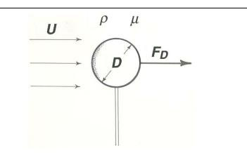
Figure 2-1. The drag force FD on a sphere moving relative to a viscous fluid.
