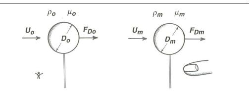
Figure 2-3. An example of scale modeling: using flows around a small sphere to model flow around a large sphere. (The object in the lower right is supposed to be someone's fingertip.)
