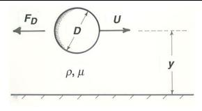
Figure 2-6. Towing a sphere parallel to a nearby solid planar wall.
