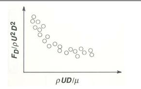
Figure 2-5. What the plot of dimensionless drag force vs. Reynolds number for flow around a sphere towed near a solid wall in a still body of water would look like if the distance of the sphere from the wall is not held constant from trial to trial.
