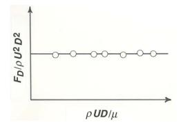
Figure 2-4. What the plot of dimensionless drag force vs. Reynolds number for flow around a sphere would look like if the viscosity were not important.
