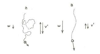
Figure 8-9. Effect of particle settling velocity relative to turbulent velocity fluctuations. **A)** The particle settles slowly relative to the vertical velocity fluctuations. **B)** The particle settles rapidly relative to the vertical velocity fluctuations.
