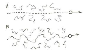
Figure 8-7. The effect of relative particle inertia when a particle moves through a turbulent fluid. A) Relative inertia is high; B) relative inertia is low.
