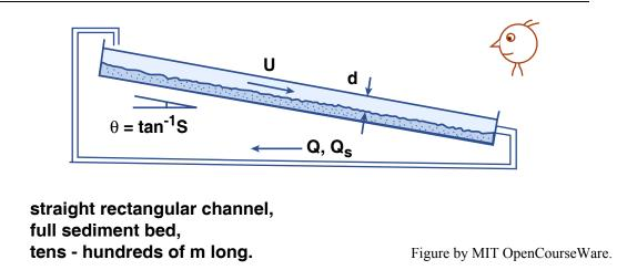
Figure 8-12. A sediment-feed flume experiment in a very short channel.
