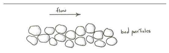
Figure 8-1. A "gravity bed" of loose sediment particles.
