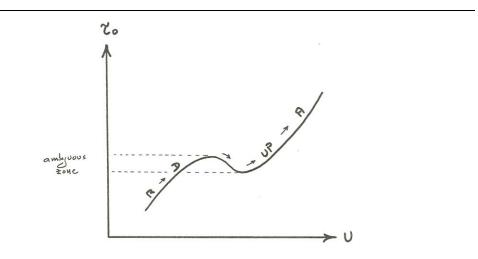
Figure 8-10. Graph of bed shear stress  $\tau_0$  vs. mean flow velocity U for a flow that is transporting sediment generating rugged bed configurations. R, ripples; D, dunes; UP, upper-regime plane bed; A, antidunes. The two horizontal dashed lines show the range of  $\tau_0$  for which a given value of  $\tau_0$  can be associated with three different values of U.
