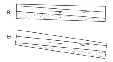
Figure 8-14. A) A uniform sediment-transporting flow in a flume with a floor that is less steep than the slope of the bed surface and the water surface. **B)** A uniform sediment-transporting flow in a flume with a floor steeper than the slope of the bed surface and the water surface.
