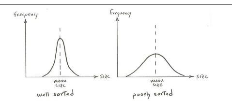
Figure 8-2. Sorting: the spread of sizes around the mean.
