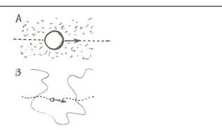
Figure 8-8. The effect of particle size relative to eddy size. A) The particles are much larger than the eddies. B) The particles are smaller than the maximum eddy size.
