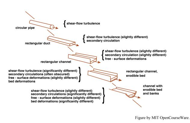
Figure 8-6. Perspective on the complexity of sediment-transporting flows.
