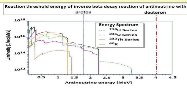
Figure. Relevance of detection threshold energy to the detection of energies of antineutrinos emitted in the decay of K, U, and Th in the Earth.
