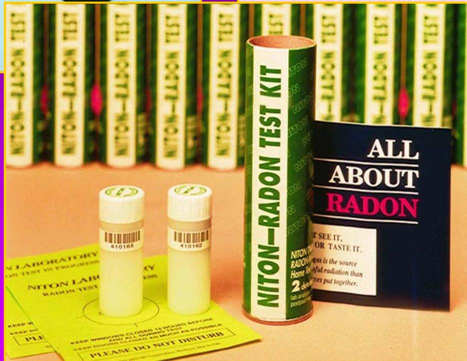
To do a screening test, place a testing device on the lowest livable level of the home for the specified testing period, remembering closed house conditions. A charcoal canister is sensitive to moisture so it should not be placed in a bathroom or kitchen where humidity may be higher.
