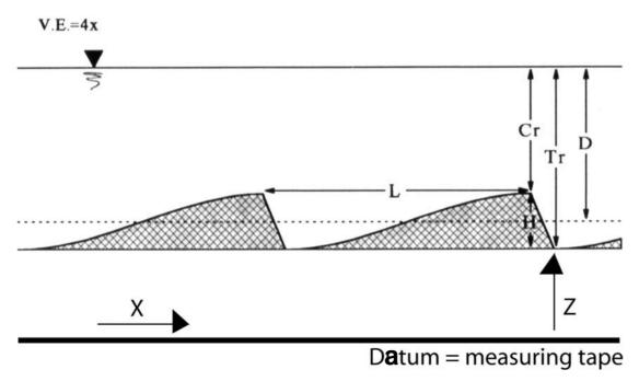
**Cr** = crest of bedform [elevation relative to some datum (e.g., the water surface)]
