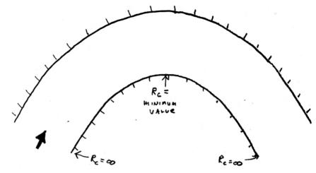
Acceleration of the fluid toward the outside bend produces a 'piling up' of fluid. This produces a cross stream slope, giving rise to a force toward the inner bank.
