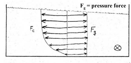
Setup of helical circulation. Force associated with surface slope is constant, centrifugal force varies with depth.
