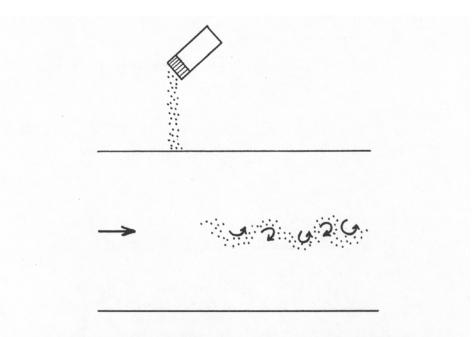
Figure 2-11 Sprinkling the flow with magic powder that allows you to see the eddies
