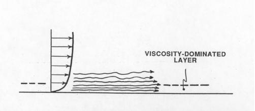
Figure 2-12 The viscosity-dominated layer at the base of a turbulent channel flow
