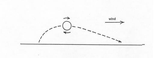
Figure 2-37 Spin of a particle saltating in air
