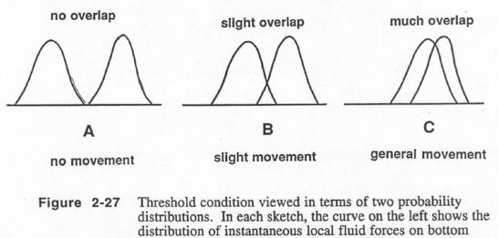
sediment particles, and the curve on the right shows the distribution of instantaneous fluid forces needed to set the bed particles in motion.
