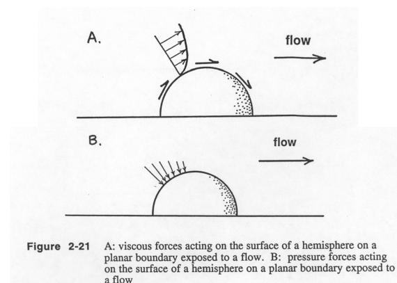
**2.2.4** Both the viscous forces and the pressure forces vary from point to point all over the surface of the hemisphere in Figure 2-20. To find the total force or resultant force exerted by the fluid on the hemisphere, you need to *sum or integrate both kinds of forces over the surface of the hemisphere*. Although this is easy to do in one's imagination, in practice it's difficult even for very large hemispheres, and it's impossible for tiny sediment particles.
