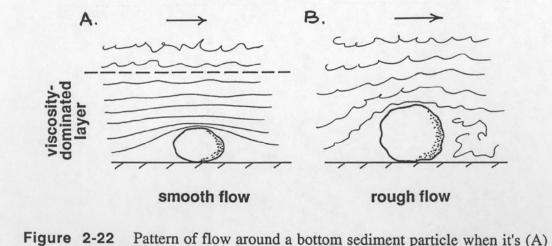
Figure 2-22 Pattern of flow around a bottom sediment particle when it's (A) embedded in the viscosity-dominated layer and (B) sticking up out of the viscosity-dominated layer
