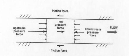
Figure 2-6 In a flow in a horizontal pipe or conduit, the fluid moves only if there's a downstream decrease in fluid pressure
