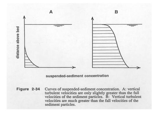
**2.4.3.7** The theory is only a qualified success, however, because the it provides only *the distribution relative to some assumed reference concentration at some reference elevation above the bed*. You can think of the bed-load layer as forming the bottom boundary condition for the suspended-sediment distribution. The key element—how the flow establishes the reference suspended-sediment concentration just outside the bed-load layer—is still not well known.
