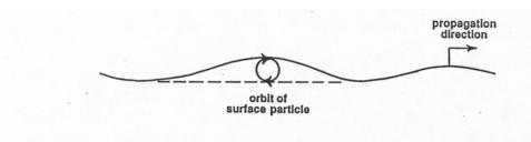
**Figure 2-16** The circular orbit of a surface particle floating on the water surface as a wave passes
