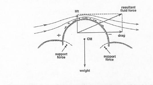
Figure 2-23 Flow and forces around a bottom sediment particle when it's embedded in the viscosity-dominated layer
