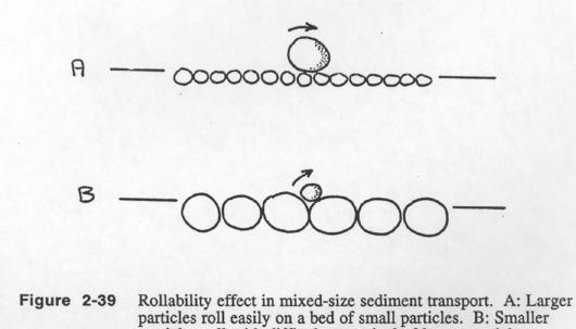
particles roll with difficulty on a bed of larger particles.
