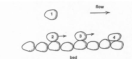
Figure 2-30 Particles that belong to the bed and that belong to the load. Particle 1 is part of the flow. Particle 2 has just come into contact with the bed but it's still moving so it's part of the flow. Particle 3 has just been set into motion, so it's part of the flow. Particle 4 is exposed to the flow but is at rest so it's part of the bed.
