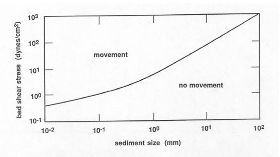
Figure 2-25 Threshold curve for incipient movement of quartz sediment in water
