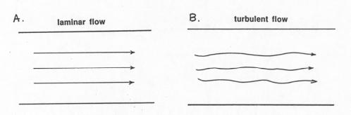
Figure 2-8 Paths of fluid elements in laminar and turbulent flow
