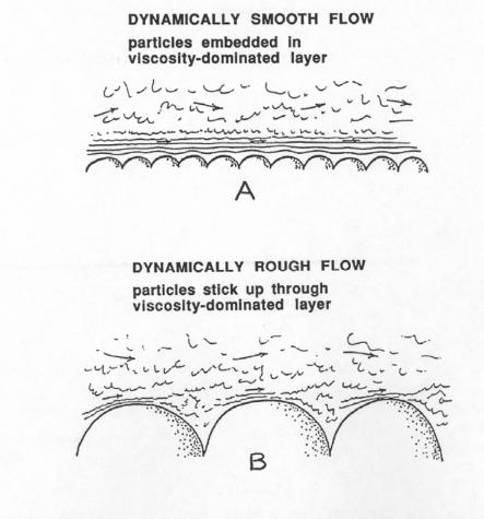
Figure 2-13 A: dynamically smooth flow B: dynamically rough flow
