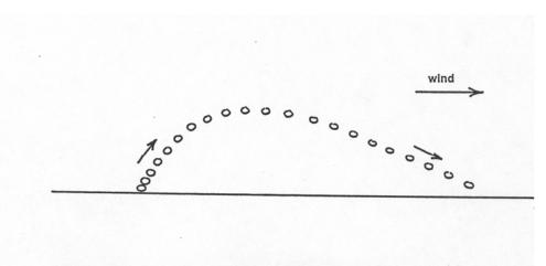
Figure 2-35 A typical saltation trajectory in air
