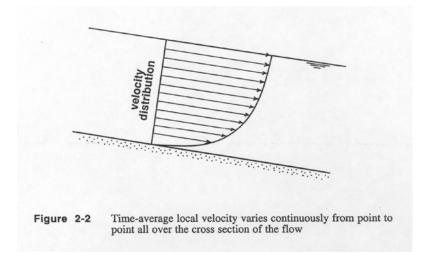
**1.2.6** You can take the average of all the local velocities all over the flow cross section to get a *mean flow velocity* U (Figure 2-3). In real rivers this is how it's actually done, but in laboratory channels, where it's easy to know the water discharge (the volume rate of flow), you can use the relationship Q = UA, where Q is the discharge and A is the area of the flow cross section, to find U.
