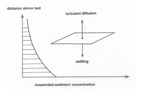
Figure 2-33 Vertical balance between downward settling and upward turbulent diffusion in suspended-load transport
