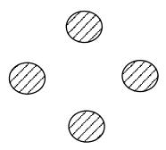
2. Imagine a beam of positive ions traveling between two poles which are positively charged. If an ion has a trajectory which carries it away from the enter, electric repulsion forces it back towards the center. Hence positively charged poles tend to have a focusing effect, keeping ions on beam.
