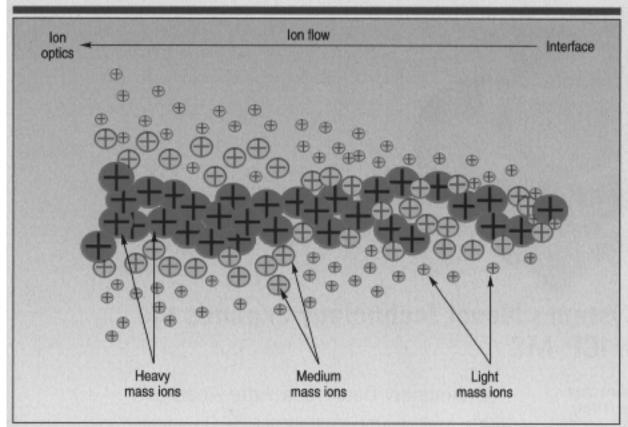
Figure 4. The degree of ion repulsion will depend on kinetic energy of the ions: those with high kinetic energy (green with red +) will be transmitted in preference to ions with medium (yellow with red +) or low kinetic energy (blue with red +).
