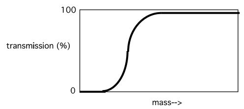
6. Suppose on the other pair of rods, an AC voltage is combined with a small negative bias. The heavy ions will tend to feel the effect of the average and be defocused and lost. The light ions will be restored to the beam by the positive phases of the AC field. Hence this pair of rods will act as a low-pass filter:
